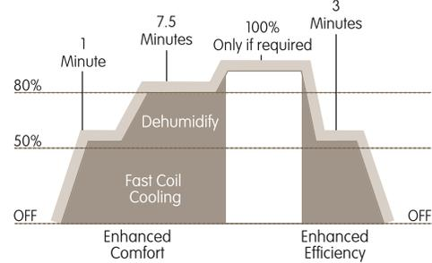
During cooling, air moves over the coil more slowly at startup, allowing the coil to rapidly cool down for increased moisture removal. This managed cycle of cooling reduces temperature variances and increases dehumidification.
