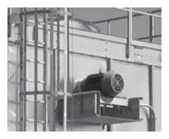
Although improved motor designs (insulation, bearings, seals, and lubricants) have now made it feasible for us to locate the motor inside the tower in close-coupled proximity to the Geareducer® (page 8), many users still prefer the motor to be located outside the humid airstream. If you are among those users—or are among those who see the wisdom of their thinking—please specify this option. If you do, however, please require it of all bidders.
