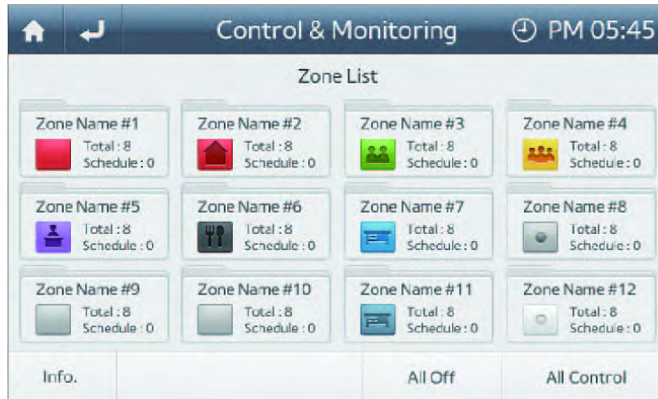
Figure 32. Control & Monitoring screen: Zone list after control option setup
