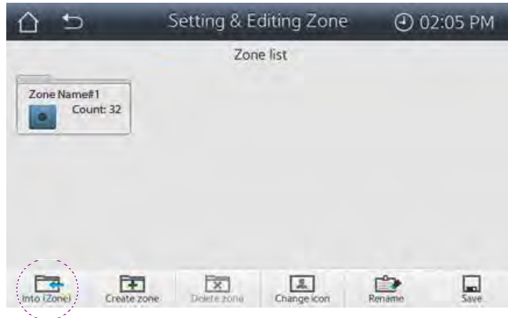
Figure 8. Setting & Editing Zone: Initial screen with a single zone containing all indoor units
